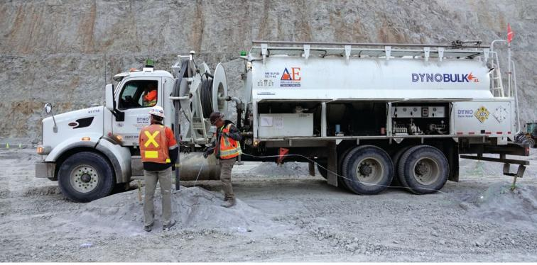
Dyno Nobel's DIFFERENTIAL ENERGY2 (ΔΕ2) allows operations to customize the explosive load in individual boreholes based on the unique geological features encountered during drilling. Photo: Dyno Nobel
